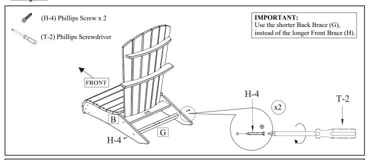
Install the shorter Back Brace (G) into the pockets of the Seat Assembly (B). Fasten using a Phillips Screw (H-4) with a Phillips Screwdriver (T-2) on each side. Do not yet fully tighten.
