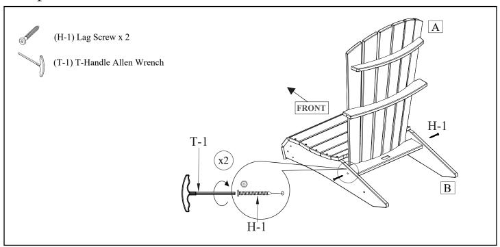
Install the Back (A) by fitting it into the pockets of the back of the Seat Assembly (B). Fasten using a Lag Screw (H-1) on each side with the T-Handle Allen Wrench (T-1). Do not yet fully tighten.
