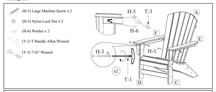
5.1 Rest the Left Arm (E) on the Left Front Leg (C) and left side of the Back Brace (A). The arm should be on the outside of the leg. Fasten the arm down using a Large Machine Screw (H-3) on the leg side and tighten using the Nylon Lock Nut (H-5) and Washer (H-6) under the arm. Tighten the screws with the T-Handle Allen Wrench (T-1) while holding the Nylon Lock Nut (H-5) in place with the 7/16" Wrench (T-3). Do not yet fully tighten. Repeat this process for the Right Arm (F).
