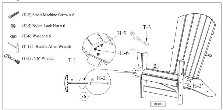
Align the three holes in the front leg assembly with the front of the Seat Assembly (B). Insert three Small Machine Screw (H-2) into the holes on each side and using the Nylon Lock Nut (H-5) and Washer (H-6) stacking the hardware in the order as shown on the inside of the seat. Tighten the screws with the T-Handle Allen Wrench (T-1) while holding Nylon Lock Nut (H-5) in place with the 7/16" Wrench (T-3). Complete for both sides.
