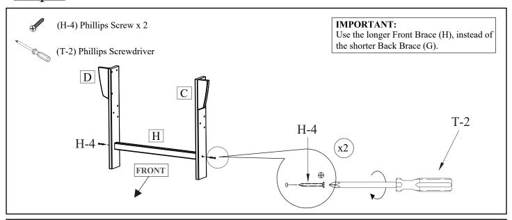
Install the longer Front Brace (H) into the Right Front Leg (D). Fasten using the Phillips Screw (H-4) with a Phillips Screwdriver (T-2). Fit the longer Front Brace (H) into the Left Front Leg (C). Fasten using the Phillips Screw (H-4) with a Phillips Screwdriver (T-2). Do not yet fully tighten.
