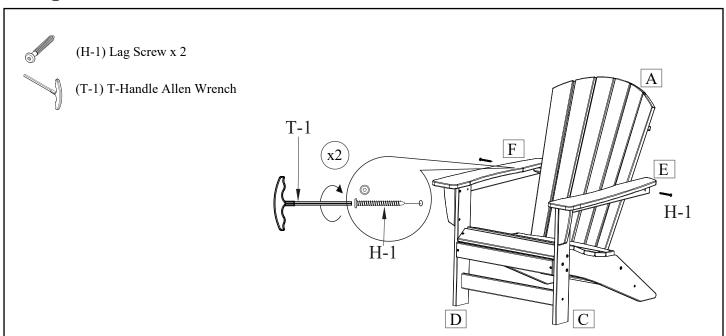
Fasten Left Arm (E) and Right Arm (F) to the Back Brace (A) using a Lag Screw (H-1) on either side with the T-Handle Allen Wrench (T-1). Fully tighten all hardware from this step and all previous steps. DO NOT OVER TIGHTEN.
